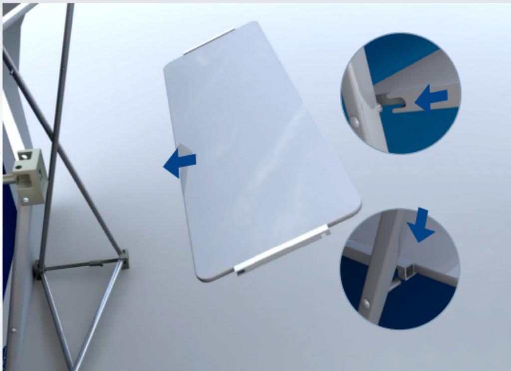
Mount the internal shelf by entering the front edge of the system's shelf fastener. Lock the shelf by allowing the rear section to fall into the system's rear shelf fastener.
